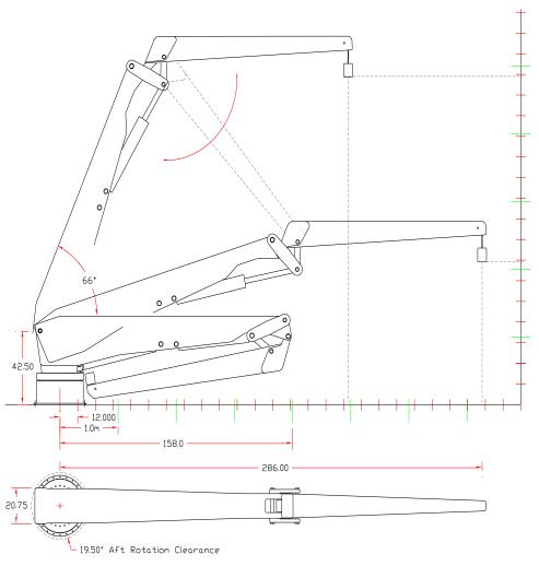
Cylindrical style pedestal bases are required and will be configured for specific applications. Floating-Flange standpipe mounting is available for GRP constructed vessels. Standpipe diameters will vary depending on the actual moment capacity of the crane.
